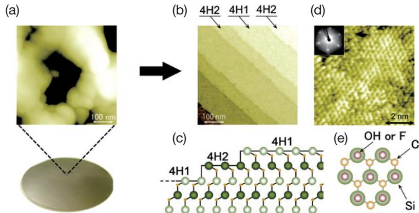
Fig. 1 (a) Unpolished 4H-SiC(0001) surface. (b) AFM image of flattened SiC surface. (c) Schematic model of 4H-SiC crystal. Deep and pale green circles represent Si atoms at cubic and hexagonal sites, respectively. Brown circles represent C atoms. (d) STM image. Electron diffraction image is superimposed. (e) Schematic drawing of OH- (or F-) terminated SiC surface.
