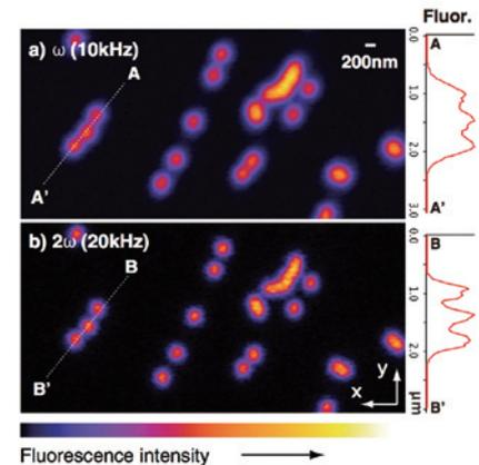
Fig. 2 The fluorescence images of fluorescence beads with a diameter of 200 nm by a) a conventional and b) the developed microscope.
