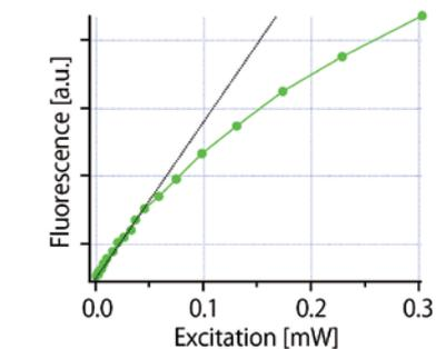
Fig. 1 The saturation effect in fluorescence excitation of Rhodamine 6G molecules.
