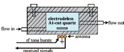
Fig. 1 Side view of the isolated electrodeless QCM cell. The line antenna is placed near the bottom of the cell, which radiates the quasistatic electric field to generate the shearing vibrations and receives the vibrational signals through the piezoelectric effect.
