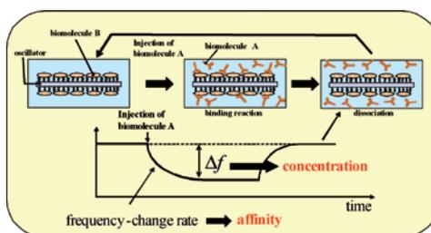
Fig. 2 Principle of the real-time monitoring of the binding and dissociating reactions between biomolecules A and B by the isolated oscillator immunosensor. The amount of the frequency change indicates the concentration of the injected protein and the frequency change rate yields their affinity.
