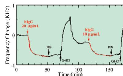
Fig. 3 Typical response of the 13th overtone resonance frequency observed during the injection sequence. IgG, PBS, and G-HCl denote the arrival times of the human IgG, phosphate-buffer solution, and glycine-HCl buffer solution, respectively.
