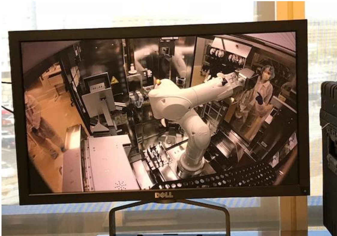
1d. Robot which retrieves medicines from storage. This robot also maintains an electronic record of amount of medicine available and expiration date of stored medicine.
