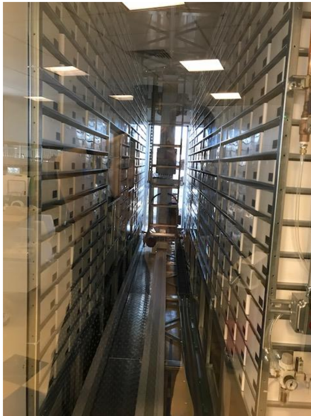
1d. Robot which retrieves medicines from storage. This robot also maintains an electronic record of amount of medicine available and expiration date of stored medicine.
